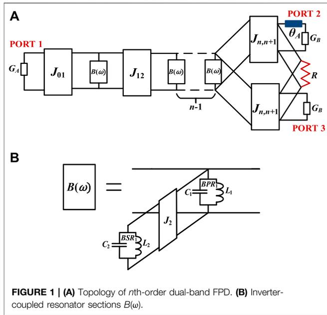
FIGURE 1 | (A) Topology of  $n$ th-order dual-band FPD. (B) Inverter-coupled resonator sections  $B(\omega)$ .
