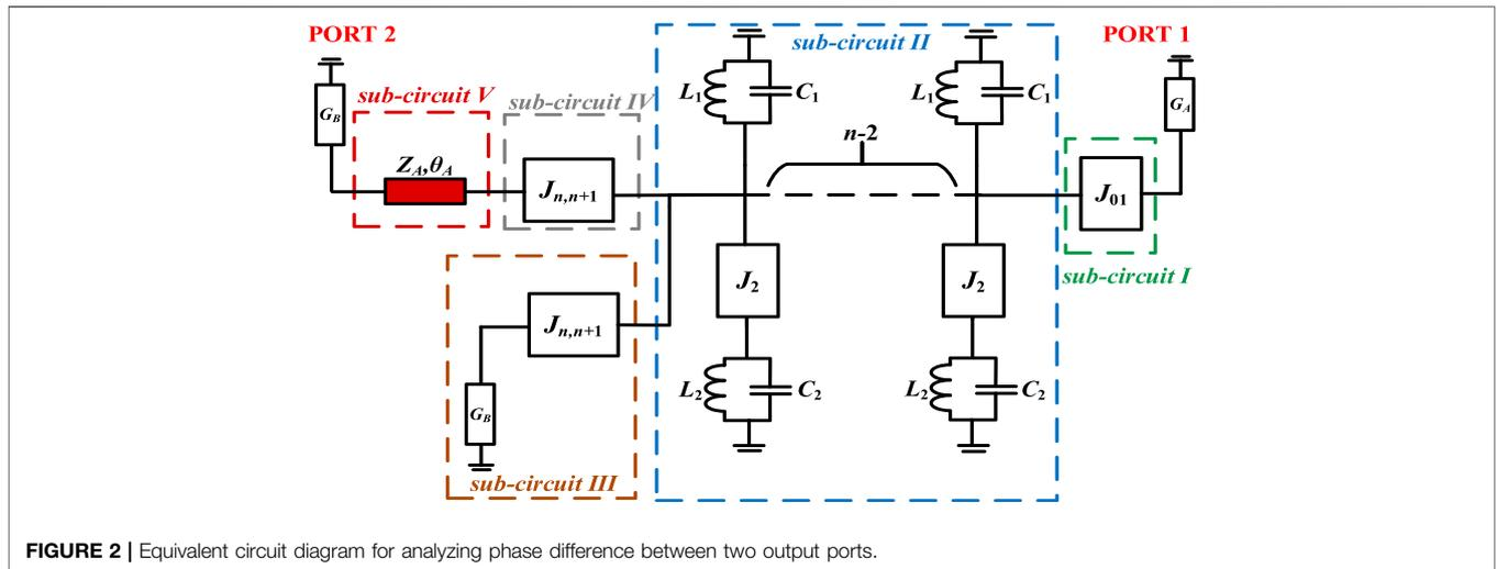
FIGURE 2 | Equivalent circuit diagram for analyzing phase difference between two output ports.
