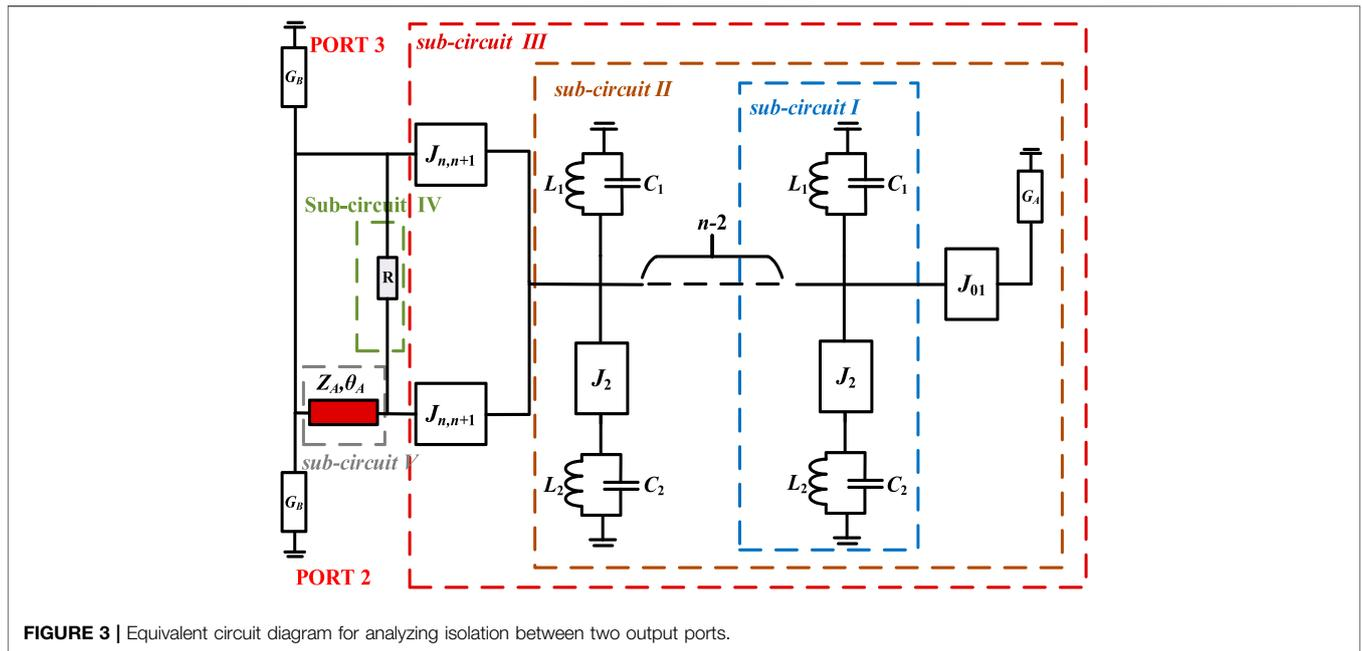
**FIGURE 3** | Equivalent circuit diagram for analyzing isolation between two output ports.
