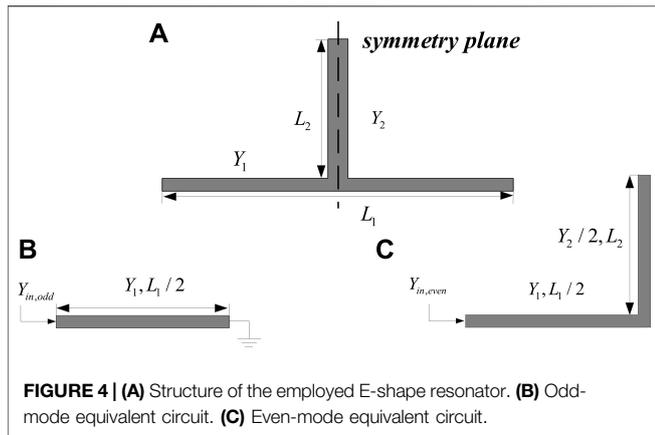
**FIGURE 4 |** (A) Structure of the employed E-shape resonator. (B) Odd-mode equivalent circuit. (C) Even-mode equivalent circuit.
