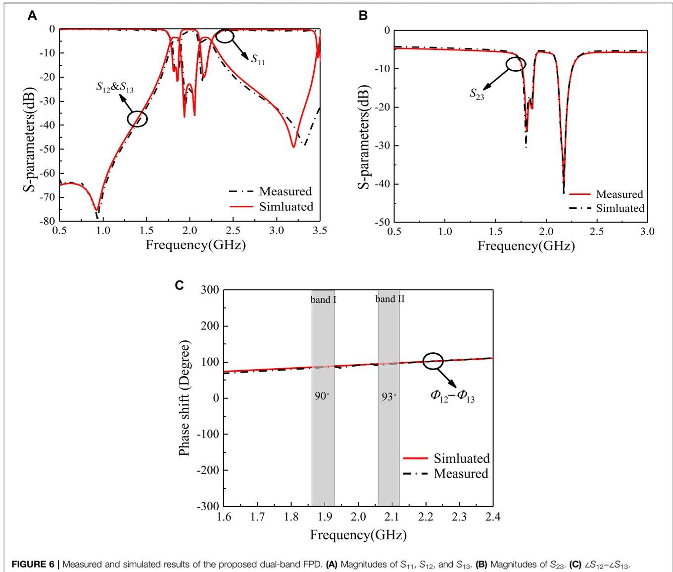
**FIGURE 6** | Measured and simulated results of the proposed dual-band FPD. **(A)** Magnitudes of  $S_{11}$ ,  $S_{12}$ , and  $S_{13}$ . **(B)** Magnitudes of  $S_{23}$ . **(C)**  $\angle S_{12} - \angle S_{13}$ .
