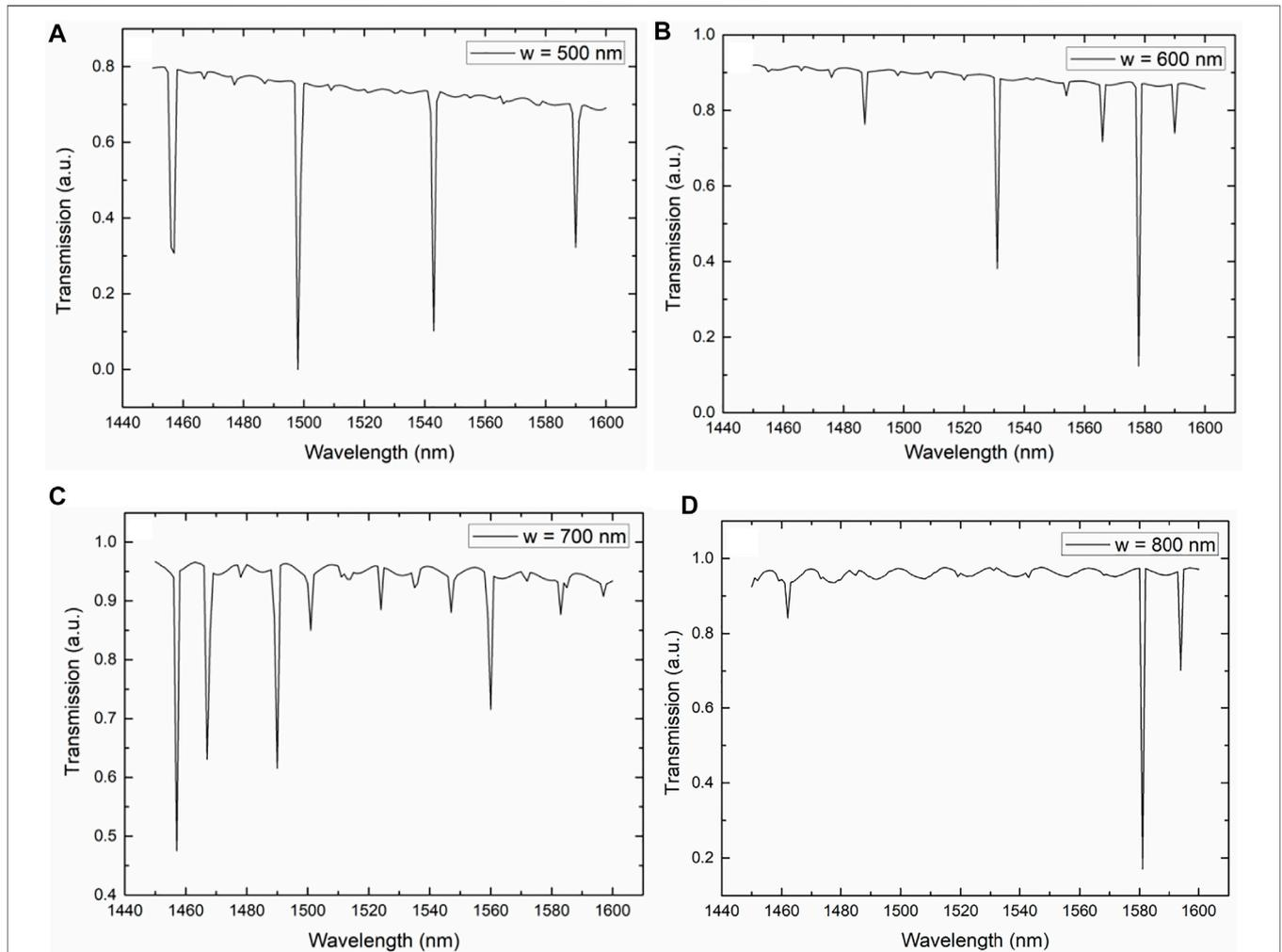
**FIGURE 5 |** Transmission curve of the sensor for different widths of the ring and waveguide varying from 500 to 800 nm by 100 nm.
