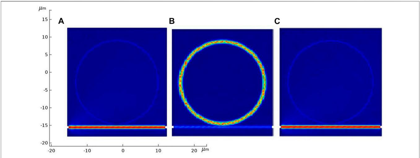
**FIGURE 3 |** Electric field distribution when the temperature is fixed at 30°C, and when the wavelength is (A) 1,542 nm, (B) 1,546 nm, or (C) 1,550 nm.
