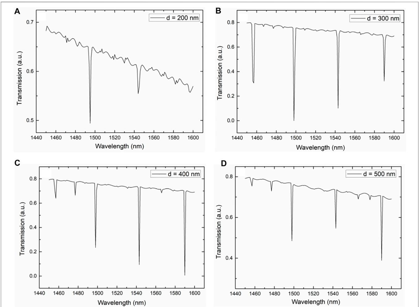
**FIGURE 4 |** Transmission curve of the device for different distances between the ring and bus waveguide varying from 200 to 500 nm by 100 nm.
