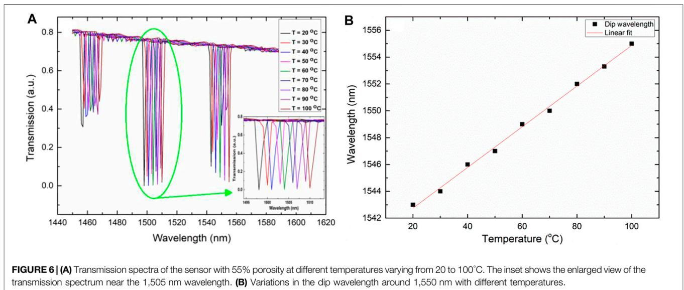
**FIGURE 6 | (A)** Transmission spectra of the sensor with 55% porosity at different temperatures varying from 20 to 100°C. The inset shows the enlarged view of the transmission spectrum near the 1,505 nm wavelength. **(B)** Variations in the dip wavelength around 1,550 nm with different temperatures.
