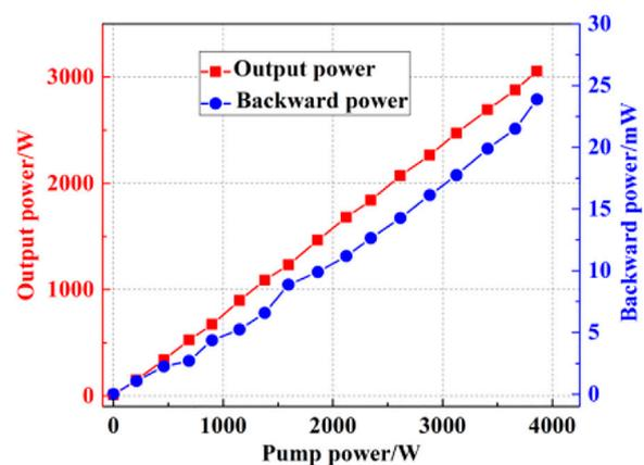
FIGURE 6 Output power and backward power versus pump power for the PM fiber laser system.
