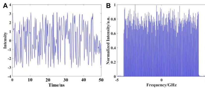
FIGURE 3 (A) Optimized phase modulation signal and (B) near-top-hat-shaped spectrum.
