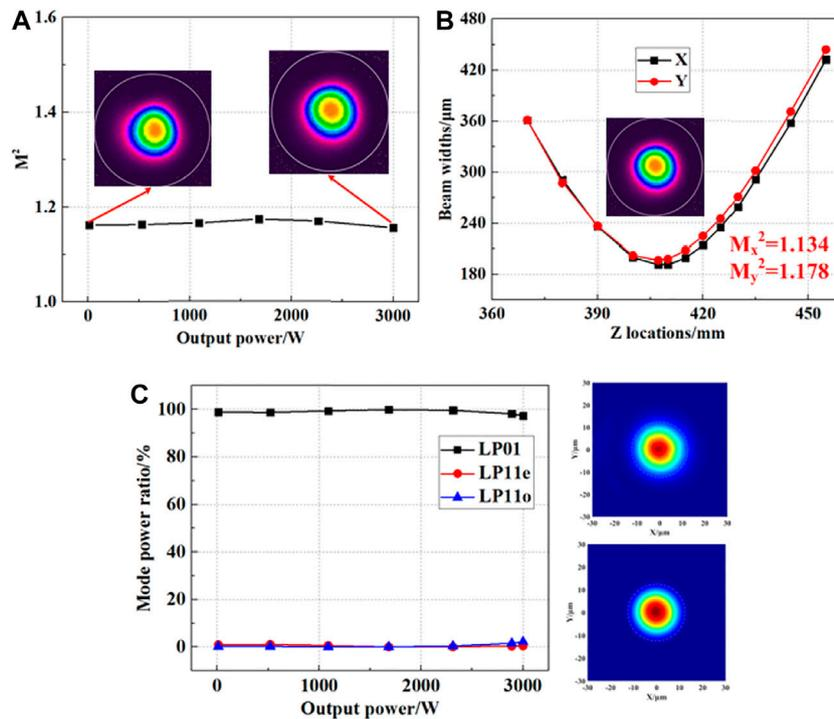
FIGURE 8 (A)  $M^2$  factors at different output powers, (B) beam quality at 3 kW, and (C) power proportion of LP01, LP11e, and LP11o modes at different output powers and the output spot (top) and mode reconstruction spot (bottom) at 3 kW.
