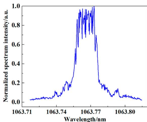
FIGURE 5 Measured normalized spectrum of the seed laser.
