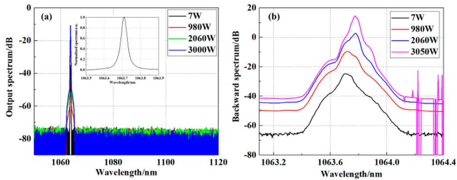
FIGURE 7 (A) Output spectrums and (B) backward spectrums at different output powers for the PM fiber laser system.
