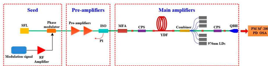
FIGURE 4 Experimental setup of the PM narrow-linewidth fiber laser (SFL, single-frequency laser; RF, radio frequency; ISO, isolator; MFA, mode field adaptor; CPS, cladding power stripper; YDF, Yb-doped fiber; QBH, quartz block head; PD, photo-detector; OSA, optical spectrum analyzer; PM, power meter).
