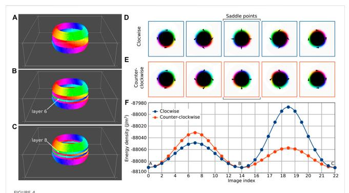
(A–C) show the normal bubble, the bubble with one alternating layer and with two alternating layers, respectively. The transitions between those bubbles require a change in the chirality of a certain layer, which can happen clockwise (D) or counterclockwise (E). (F) Contains four minimum energy paths corresponding to transitions (A, B) and (B, C). Saddle points have a Neel bubble shape in all cases.
