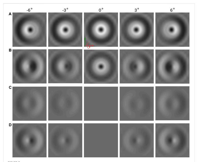
Lorentz TEM images of magnetic bubbles with different domain wall structures at different tilt angles of the incident electron beam. Each row of images corresponds to a particular type of bubble domain depicted in Figure 2: (A) normal bubble with fixed chirality across all internal layers, (B) bubble domain in the presence of weak iDMI, (C) bubble domain at strong iDMI, and (D) bubble domain with alternate chirality across the internal layers.
