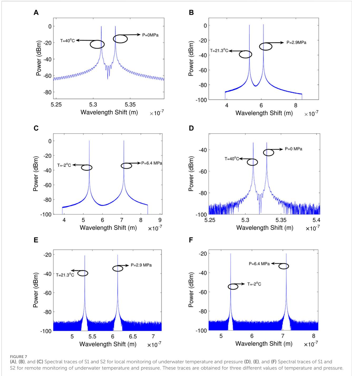
that a combined temperature and pressure can be simulated and sensed. This process can be designed using the sensitivity (slope) parameter of the sensors. The reflected optical signals from sensors at shifted Bragg wavelengths corresponding to the swept values of the temperature and pressure in the range of 40 to  $-2^{\circ}\text{C}$  and 0–7 MPa, respectively are combined using 5:95 cross coupler (x-coupler) which is basically a fused optical coupler (FOC).
