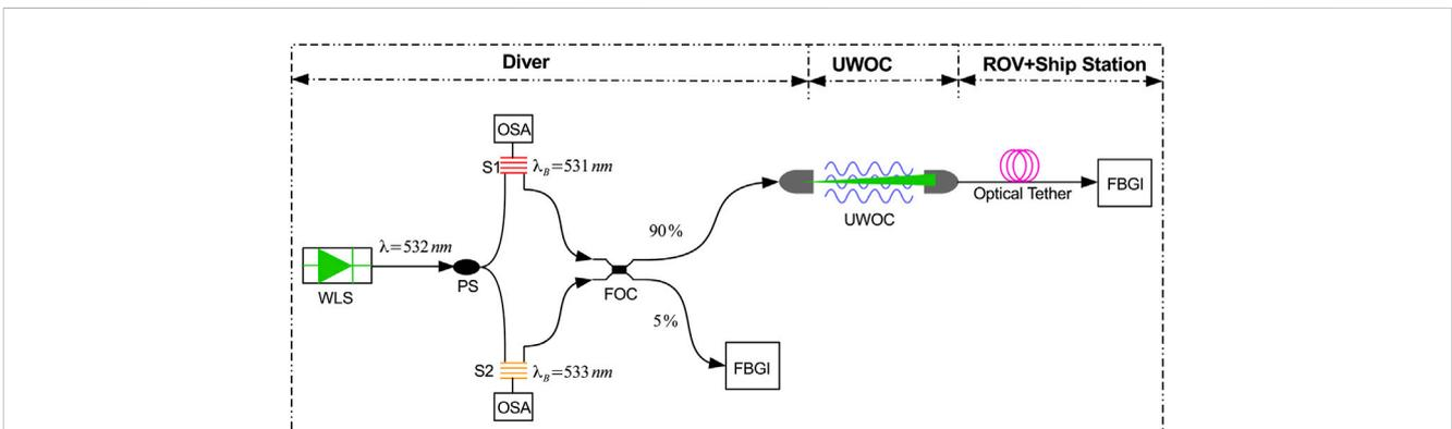
FIGURE 3 Block diagram of the proposed setup, WLS: White light source, PS: Power splitter, S: FBG sensor, FOC: Fused optical coupler, UWOC: Underwater optical communication channel, FBGI: Fiber Bragg grating interrogator, OSA: Optical spectrum analyzer.
