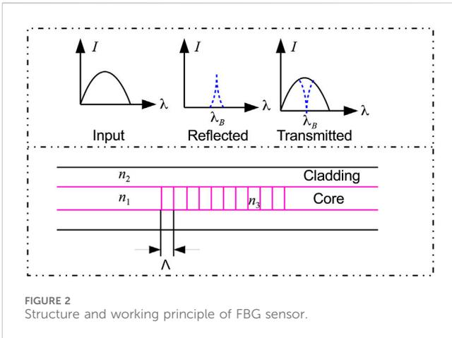
FIGURE 2 Structure and working principle of FBG sensor.
