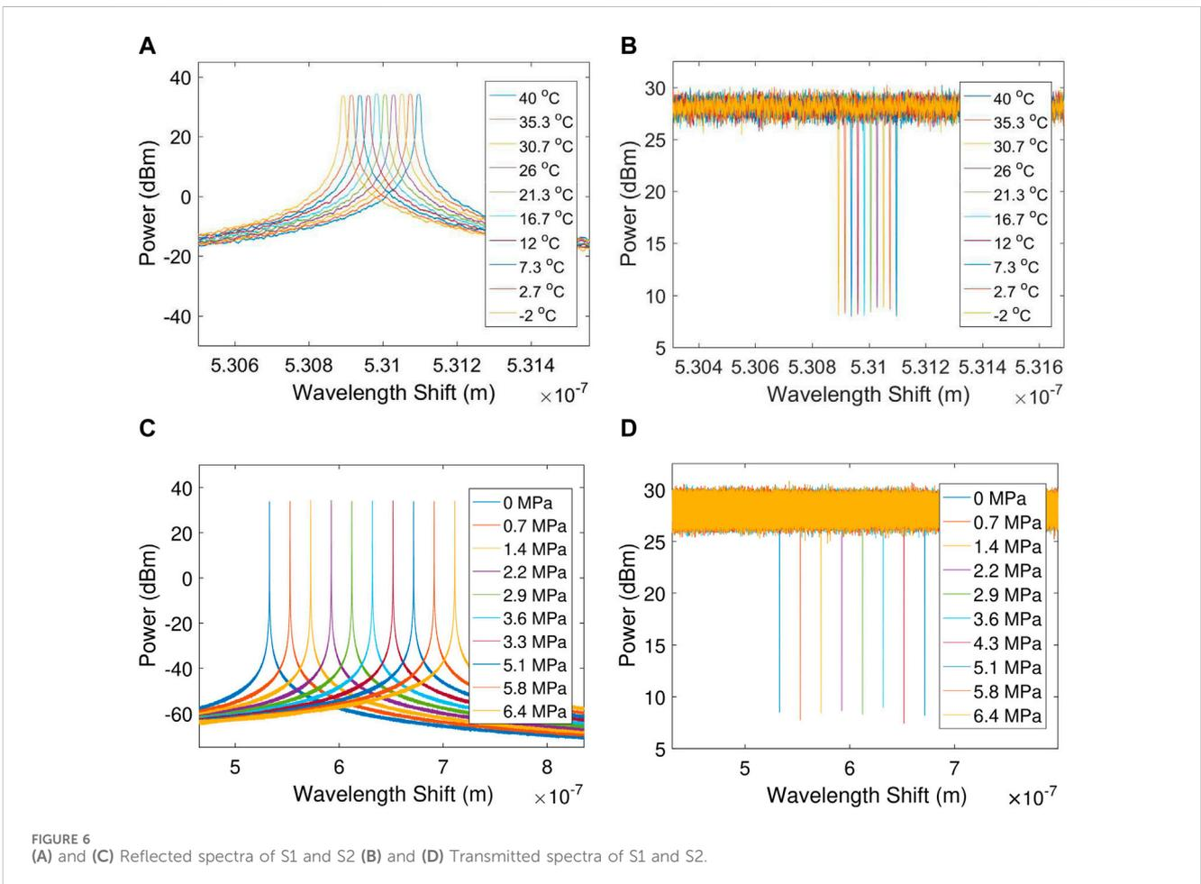
Oceanic and Atmospheric Administration (NOAA) [27]. The effect of pressure on the wavelength shift of the S2 is much more compared to the variation due to the temperature. Typically, there might be an overlap between both effects on the wavelength shift of the sensors that causes ambiguity. However, using calibration tables and proper choice of the center wavelength of sensors, it is possible to synthesize the effect when both temperature and pressure produce any wavelength shift and
