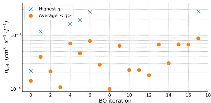
FIGURE 8 Fusion parameter  $\eta_{\text{net}}$  as a function of the BO iteration for all simulations.
