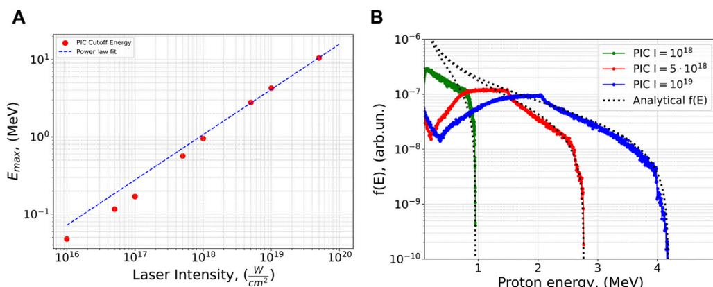
FIGURE 4 (A) PIC cutoff energies and power law fit for a cluster with  $r = 50$  nm and  $n_0 = 100 n_{crit}$ . (B) Normalized PIC proton energy spectrum for various laser intensities  $I$  and analytical probability density function (PDF) based on equations derived by [39].
