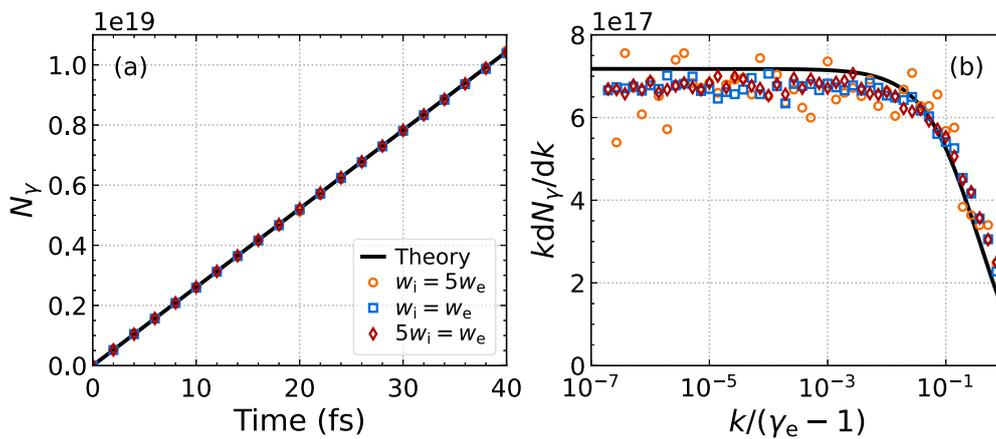
**FIGURE 4** Bremsstrahlung emission from a 1-MeV electron beam incident on solid-density boron. The simulation results (markers) match the theoretical predictions (black curve) for the (A) total photon count and (B) normalized photon energy spectra independent of the ratio of the weights of the electron and ion macroparticles.
