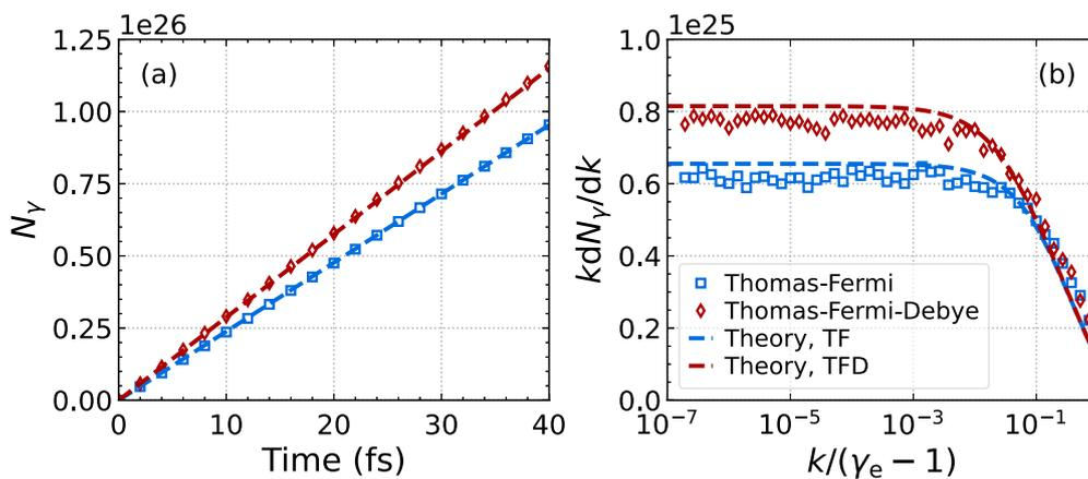
**FIGURE 5** Bremsstrahlung emission from 1-MeV electrons in a charge-neutral fully ionized boron plasma at 200 keV and 1,000 g/cm<sup>3</sup>. Plotted are the simulated (markers) and expected (curves) (A) photon count and (B) normalized photon energy spectra for the combined Thomas-Fermi-Debye Coulomb potential model (red) and single Thomas-Fermi potential model (blue).
