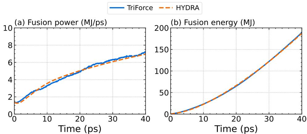
FIGURE 11 (A) Fusion power and (B) total fusion energy produced from the DT hot-spot simulated with TRIFORCE (blue) and HYDRA (orange).
