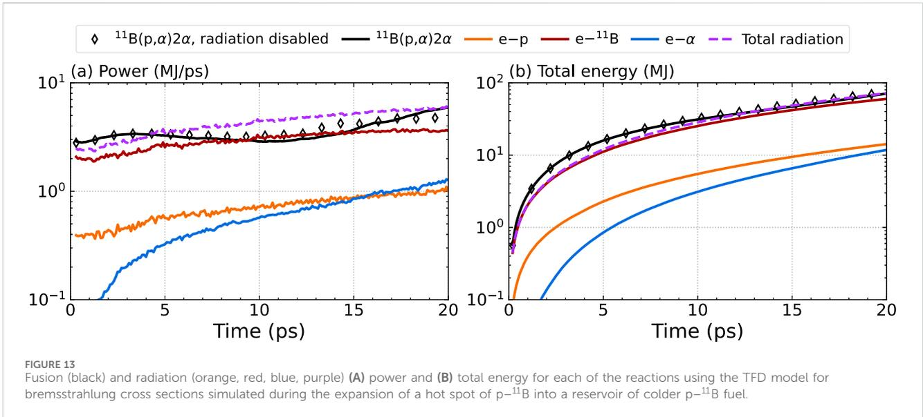
channels is 71.7 MJ. When the radiation model is disabled, the integrated fusion energy after 20 ps is 73.4 MJ. The model predicts only a small decrease in net fusion energy in the simulated time because most of the radiated photons are re-absorbed by the high-density opaque plasma. If radiation absorption is not included in the model, the predicted fusion power drops below 1 MJ/ps due to radiative losses.
