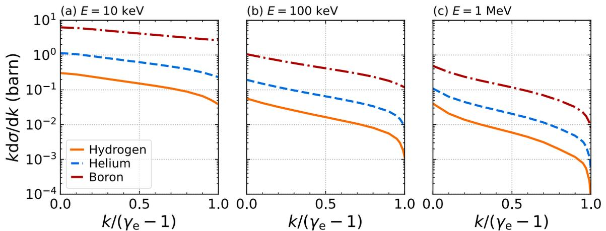
**FIGURE 2** Bremsstrahlung differential cross sections as a function of  $k/(\gamma_e - 1)$ , the emitted photon energy normalized to the electron energy, for atomic numbers  $Z = 1, 2,$  and  $5$  are shown for electron–nucleus interactions with energies equal to (A) 10 keV, (B) 100 keV, and (C) 1 MeV. Cross-section tables based on Seltzer and Berger data [35] were collected from the Geant4 database [36–38].
