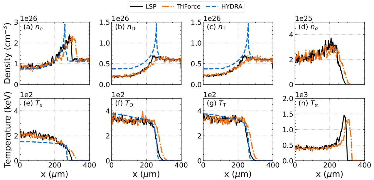
**FIGURE 9** Simulated expansion of a 30-keV DT hot-spot into cold fuel at 40 ps simulated with LSP (black), TRIFORCE (orange), and HYDRA (blue). Plots (A-D) show density and plots (E-H) show temperature for the electron, deuterium, tritium, and alpha plasma species. Some smoothing is applied to the results from the particle codes.
