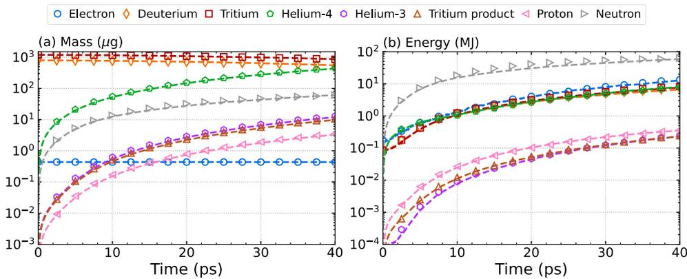
**FIGURE 10** The total mass and energy as a function of time for the simulated release of 30-keV DT into cold DT including Coulomb collisions and fusion reactions between D–D, D–T, and D–<sup>3</sup>He. Shown are the (A) integrated mass and (B) kinetic energy for each of the plasma species simulated with TRIFORCE (markers) and LSP (curves).
