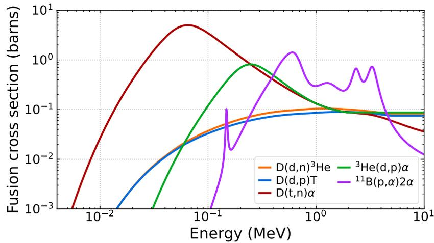
FIGURE 1 Fusion cross sections as a function of the center-of-mass energy from Bosch and Hale [3], the International Atomic Energy Agency Evaluated Nuclear Data File [4], and Tentori and Belloni [5].
