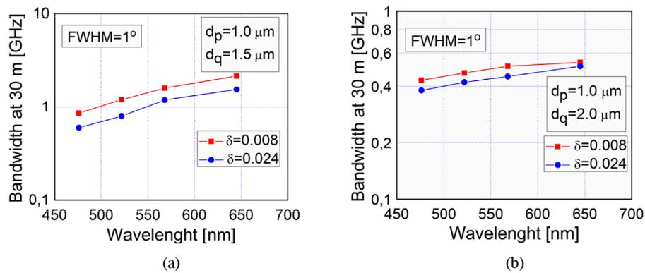
**FIGURE 2** Calculated bandwidth at 30 m vs. wavelength for W-type mPOF with  $\delta = 0.008$  and  $0.024$ , and  $d_p = 1 \mu\text{m}$ , for Gaussian beam excitation with FWHM =  $1^\circ$ , (A)  $d_q = 1.5 \mu\text{m}$  and (B)  $d_q = 2 \mu\text{m}$ .
