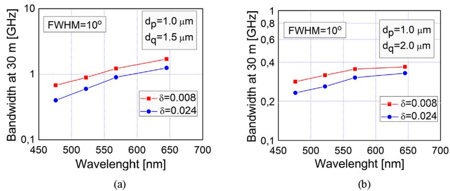
**FIGURE 3** Calculated bandwidth at 30 m vs. wavelength for W-type mPOF with  $\delta = 0.008$  and  $0.024$ , and  $d_p = 1 \mu\text{m}$ , for Gaussian beam excitation with FWHM =  $10^\circ$ , (A)  $d_q = 1.5 \mu\text{m}$  and (B)  $d_q = 2 \mu\text{m}$ .
