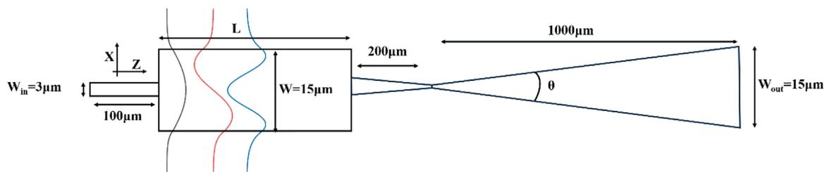
FIGURE 1 Schematic diagram of the waveguide structure of the new tapered semiconductor laser with integrated multimode interference coupler.
