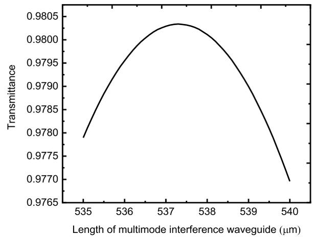
FIGURE 6 The relationship between the transmittance of the new semiconductor tapered laser and the length of multimode interference waveguide.
