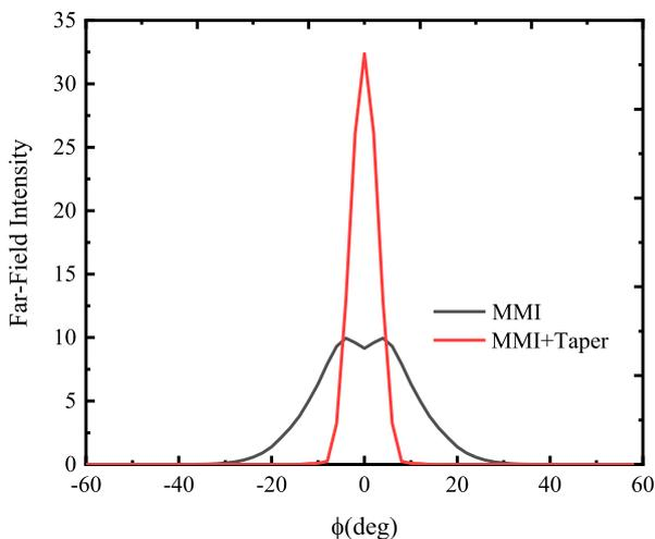
FIGURE 5 Comparison of the far-field distribution between conventional MMI laser and new semiconductor tapered laser.
