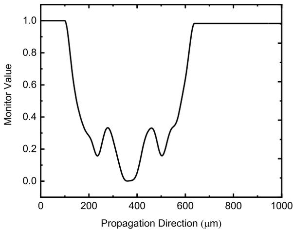
FIGURE 4 The total field strength in a region of 3 μm equal width to the input waveguide along the 1 × 1 MMI z-axis.
