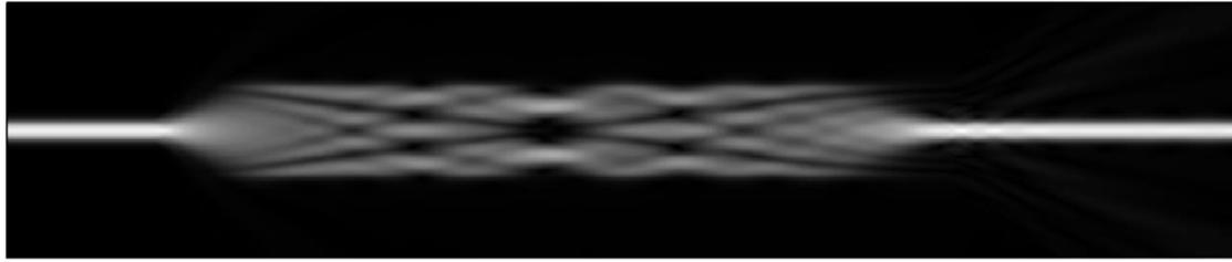
FIGURE 3 Diagram of the field distribution in 1 × 1 MMI.
