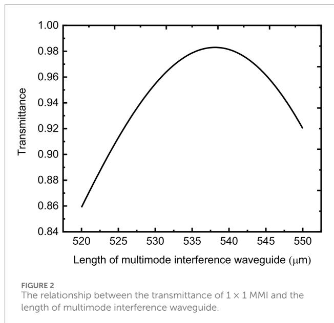
FIGURE 2 The relationship between the transmittance of  $1 \times 1$  MMI and the length of multimode interference waveguide.
