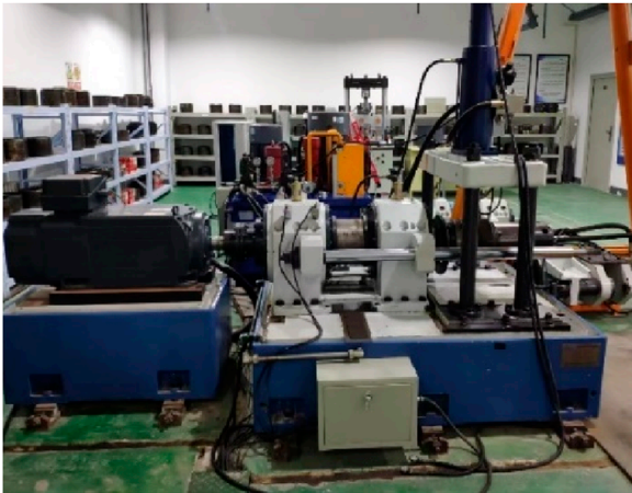
FIGURE 4 Photograph of the wheelset bearing test platform.
