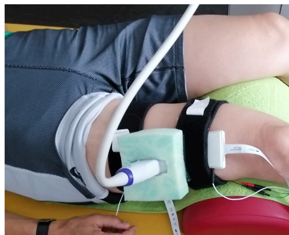
FIGURE 1 The ultrasound transducer was hosted in a custom-cut foam block, here for recording the M. vastus lateralis.
