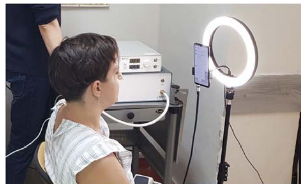
FIGURE 1 Location and setup of the measurements. The subject sat with the back supported. The phone was mounted on a tripod at head level with an LED lamp in the background.
