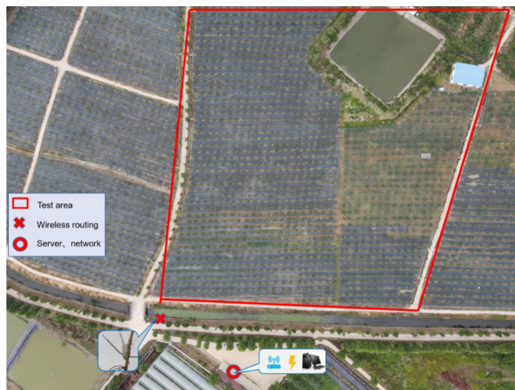
FIGURE 10 Aerial view of the Pear Garden. The red circle shows one of the houses in the pearly gardens, where power and internet are provided and where the server for the experiment was placed. The quadrilateral box represents the area for this experiment. The location of the crosses is the outdoor router.
