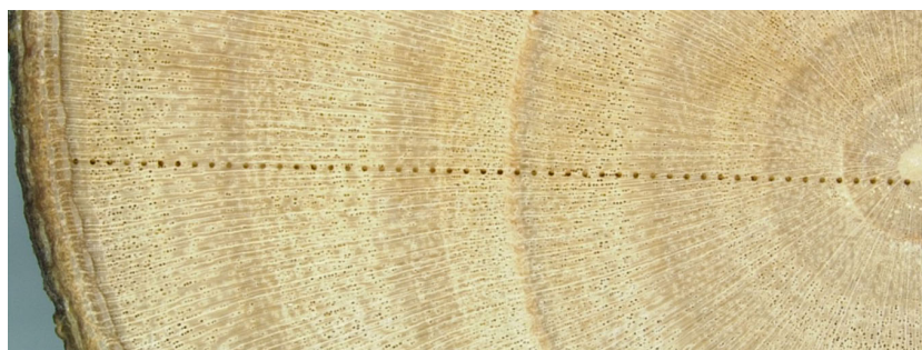
FIGURE 1 Laser shots (100 \mu m) spaced 300 \mu m apart in a magnified cross-section of an olive tree branch from the cultivar Arbosana.
