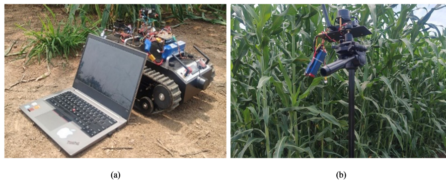
FIGURE 3 Field test environment and platform. (a) TR400 field test platform. (b) Navigation system base station.
