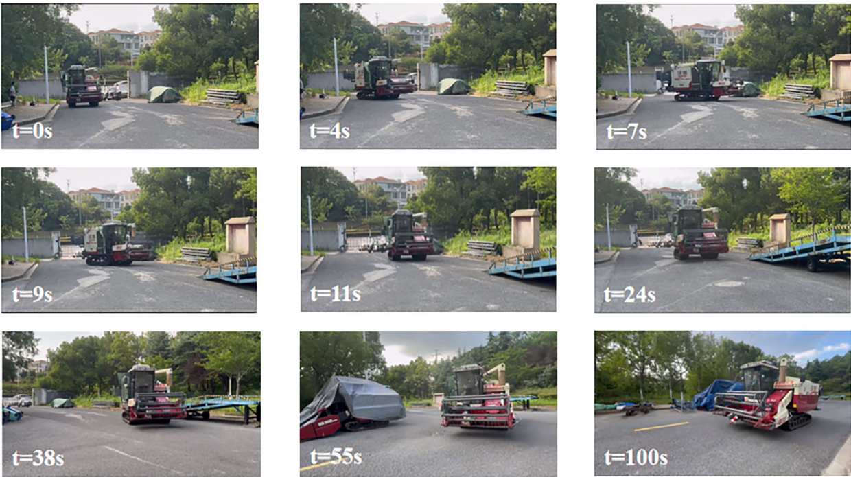
FIGURE 15 Combine harvester path tracking process.
