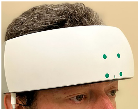
FIGURE 4 fNIRS apparatus. The NIRSIT near-infrared spectroscopy device (shown on the head of a researcher) was positioned on the forehead, centered on the midsagittal line, and secured with a Velcro strap.
