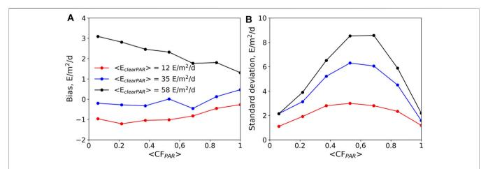
FIGURE 3 | Algorithm uncertainity on individual < E\_PAR > estimates (i.e., using one observation per day) as a function of < CF\_PAR > for several values of < E\_clearPAR > . (A) Bias (estimated minus simulated values); (B) standard deviation. The theoritical uncertainity was obtained from simulations of the TOA reflectance and <E<sub>PAB</sub>>for a wide range of situations using 10 years of MERRA-2 aerosol and cloud data (see text for details).
