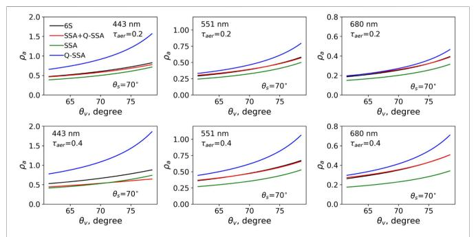
**FIGURE 1** Atmospheric reflectance  $\rho_a$  parameterization using SSA, Q-SSA, and a combination of SSA and Q-SSA (green, blue, and black dots, respectively). 6S calculations (RT) are displayed as red curves. Sun zenith angle is 70 deg., scattering angle is 171.5 deg., aerosols are of maritime type with optical thickness of 0.2 and 0.4 at 550 nm, and wavelengths are 388, 551, and 680 nm.
