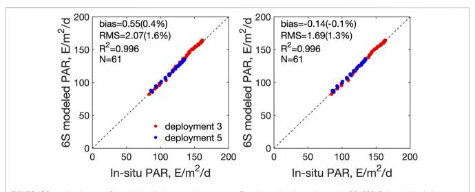
FIGURE 6 | Comparison between 6S-modeled and field-measured instantaneous < EPAR> in very clear sky conditions at the BOUSSOLE site using hourly data: (Left) before any correction; (Right) after adjustment of the measured values to the 6S value via linear regression.
