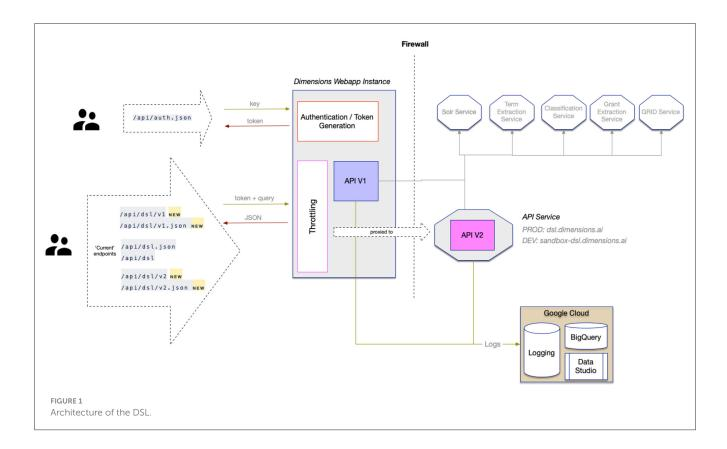
contains all the necessary data to build a final Solr query, such as information about which fields to return and what filters to apply, what facets to compute, etc. The intermediate representation is then validated against configured mappings and configuration, authorizations calculated, optimized, and only then translated to the final representation.
