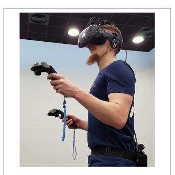
FIGURE 4 | User equipped with the required devices for the experiment: HTC Vive virtual reality headset, Vive trackers, TP Cast wireless adapter. Written informed consent was obtained from the depicted individual for the publication of this image.
