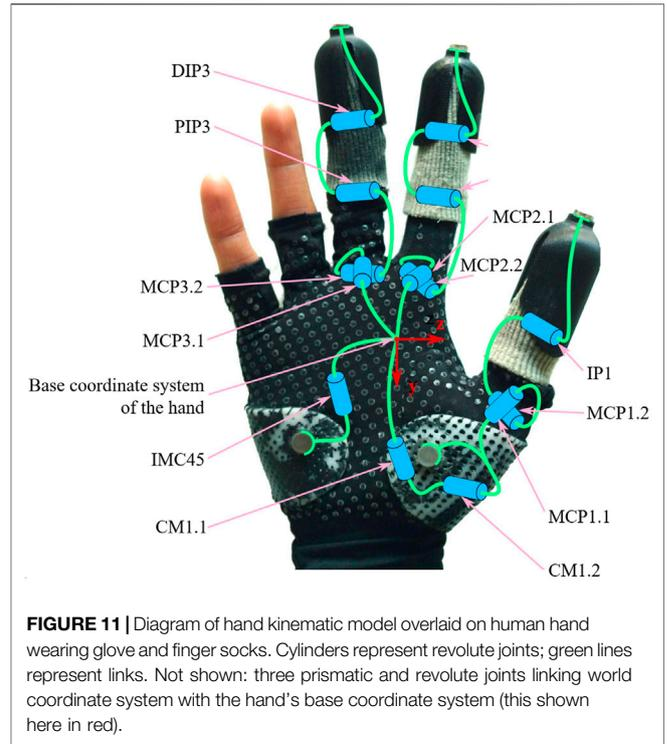
**FIGURE 11** | Diagram of hand kinematic model overlaid on human hand wearing glove and finger socks. Cylinders represent revolute joints; green lines represent links. Not shown: three prismatic and revolute joints linking world coordinate system with the hand's base coordinate system (this shown here in red).
