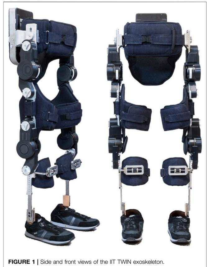
**FIGURE 1** | Side and front views of the IIT TWIN exoskeleton.
