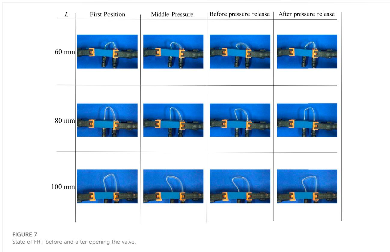
In addition, a metal plate was bound together with the urethane tubes to maintain a constant thickness when the urethane tube was flattened.
