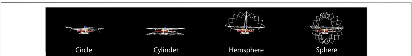
**FIGURE 11** | We designed four varieties of expandable structures for PufferBot, each with trade-offs in the amount of protection it can provide, visual saliency for communication purposes, and weight.
