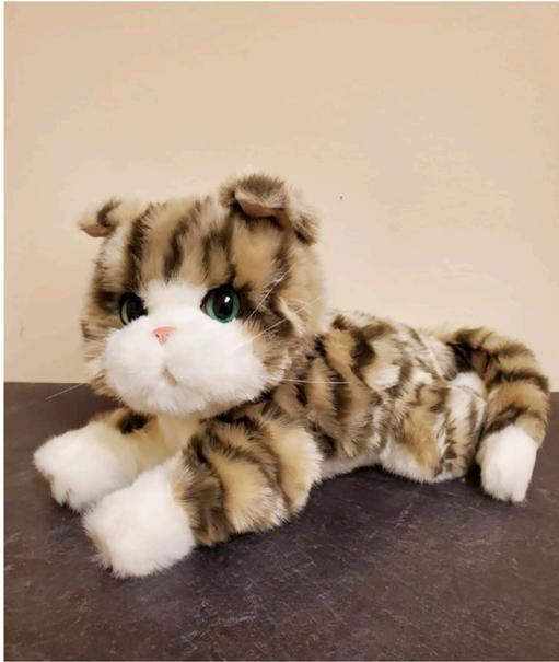
**FIGURE 1 |** Joy for All robot kitten. The robot kitten has soft faux-fur, purrs (vibrates) using a technology the company refers to as VibraPurr, and kneads (i.e., moves its front paws up and down). The robot kitten weighs about 1 pound and takes three AA batteries.
