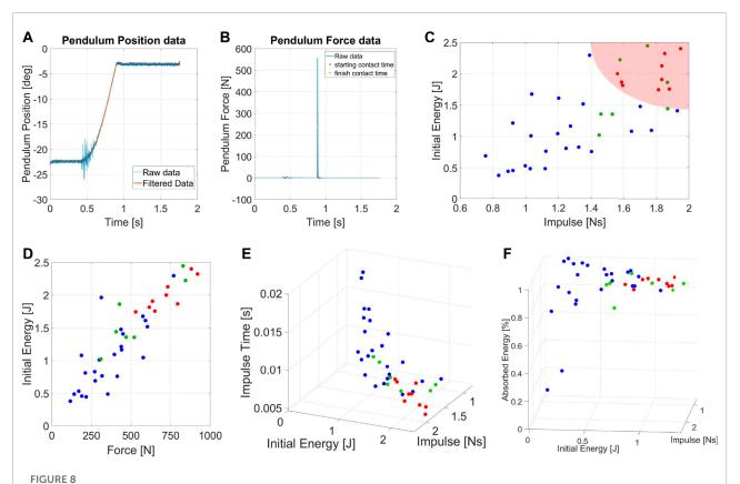
Measurement of (A) angular position and (B) force sensor data for the impulsive experiments. (C) Chart of the IRfor the Humanoid robot Alter-Ego. (D) Forces resulting from the impulsive tests applied Alter-Ego. (E) Impulse Time of the experiments varying the initial conditions. (F) Chart of the AEIfor the Humanoid robot Alter-Ego.
