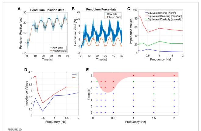
Measurement of (A) angular position and (B) force estimation for the sinusoidal force disturbance experiments. The used condition for the test are f = 0.1Hz and  $A_F = 3N$ . (C) EEland (D) Equivalent damping ratio ( $\epsilon$ ) and natural frequency ( $\omega_n$ ) related to sinusoidal force protocols. (E) Chart of the ERrelated to repetitive forces for Alter-Ego.
