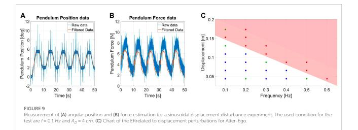
ERreveals a low-frequency force range which is more destabilizing for Alter-Ego. Its dynamics act as a low pass filter, better rejecting high-frequency perturbations. In case of repetitive displacement perturbations, the pendulum provides faster and stronger pushes at higher frequencies, resulting in the robot that eventually falls when the frequency exceeds
