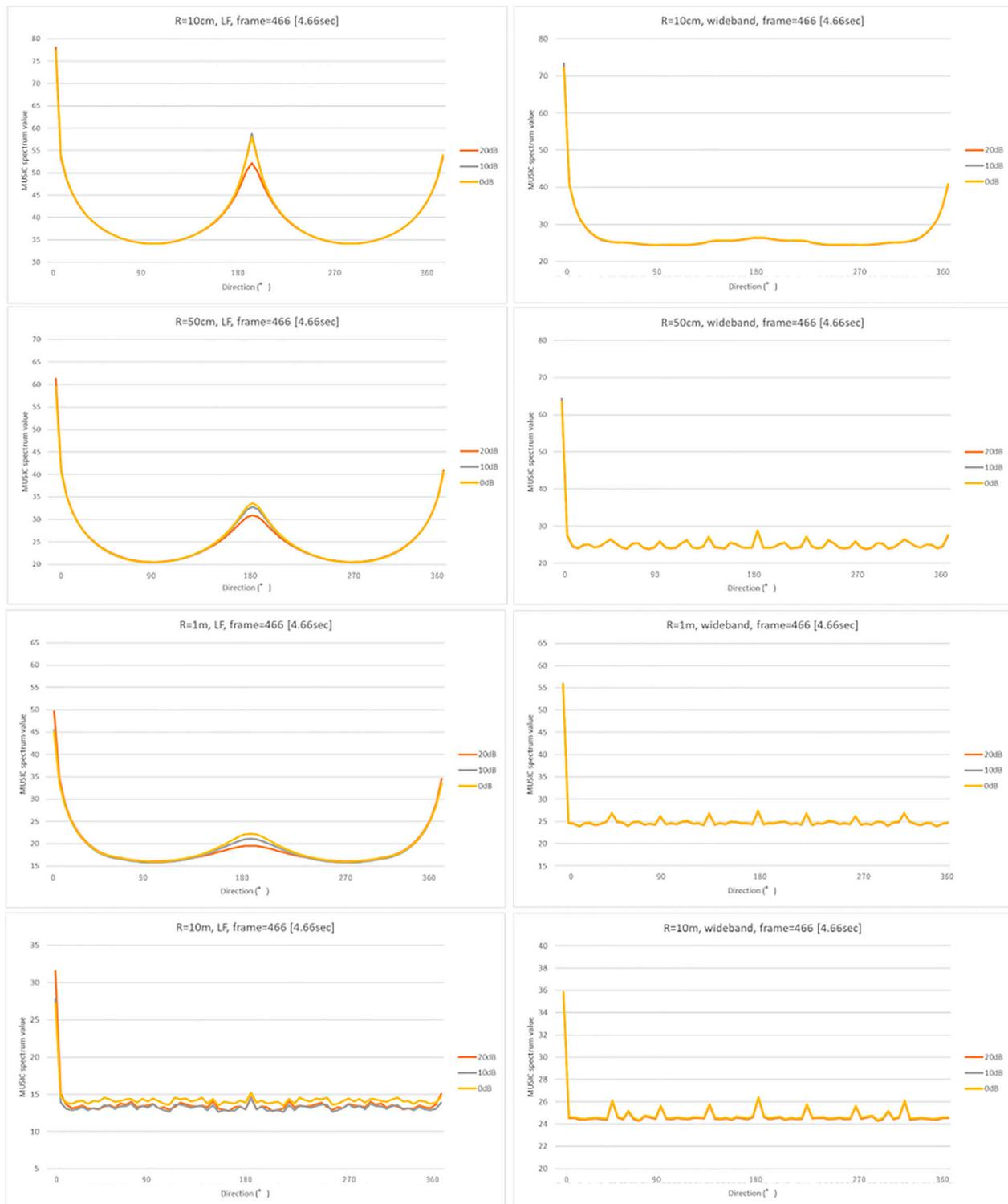
**FIGURE 6 |** MUSIC spatial spectrum for LB (left) and WB (right). The vertical and horizontal axes indicate the direction and MUSIC spatial spectrum value, respectively. The conditions of the 1<sup>st</sup>-4<sup>th</sup> subgraphs correspond to those of the 2<sup>nd</sup>-5<sup>th</sup> subgraphs in **Figure 5**.
