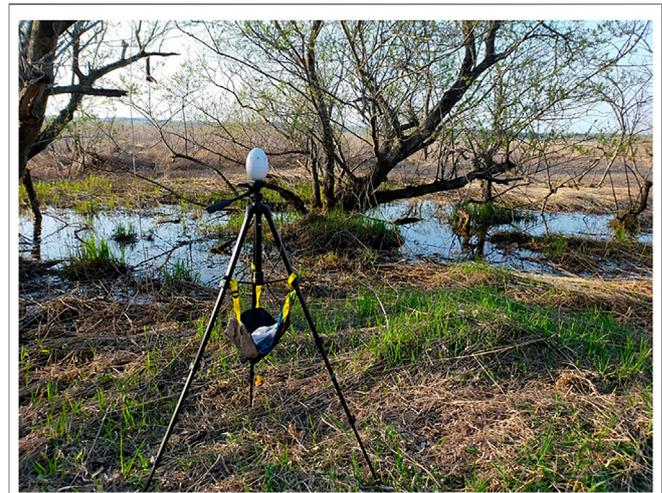
**FIGURE 4** | Photograph of the 8-channel microphone array.
