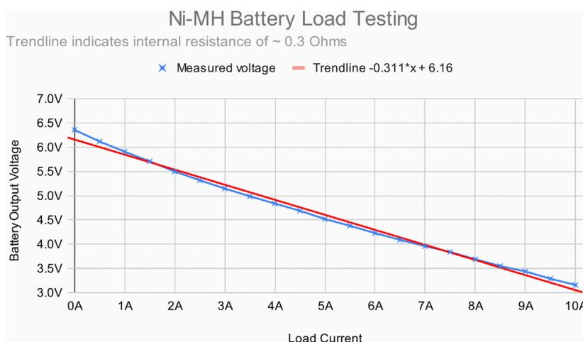
**FIGURE 10** The output voltage measured across the terminals of the 5-cell Ni-MH battery at different load currents. The gradient of the current-voltage line indicates the internal resistance of the battery, approximately 0.3 Ω.
