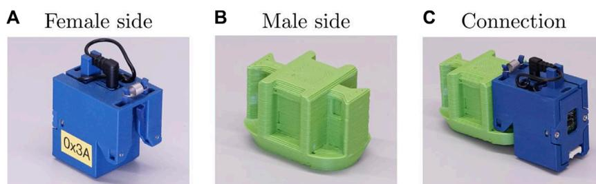
**FIGURE 5** This figure shows the mechanical connector used in the ARE platform. The female side (A) uses two sprung arms to engage with the indentations on the male side (B) to form the final connection (C).
