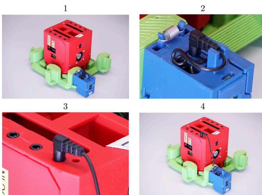
**FIGURE 6** Retractable cables are used to interconnect organs, shown here at the different stages of the connection process: 1) The organ is clipped onto the skeleton. 2) The retractable cable is drawn out from a cavity in the organ casing. 3) The cable is connected to the head. 4) The coiled cable self-adjusts its length to the distance between the head and the organ.
