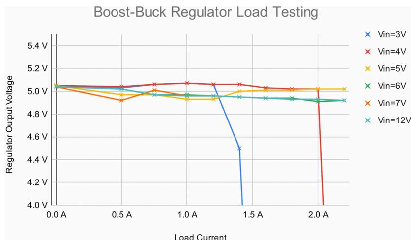
**FIGURE 11** The output voltage measured at the output of the boost-buck regulator circuit at different load currents and input voltages, showing that it can easily step down from higher voltages, but the extra switch current required in boost mode limits how low the input voltage can go. Sudden drops indicate thermal cutout of the regulator, showing the limits of its output capability.
