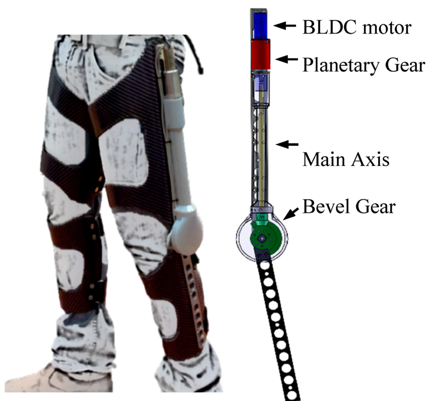
FIGURE 1 Mechanical design of the autonomous energy exoskeleton mounted on the knee brace (reproduced from Gad et al., 2022).
