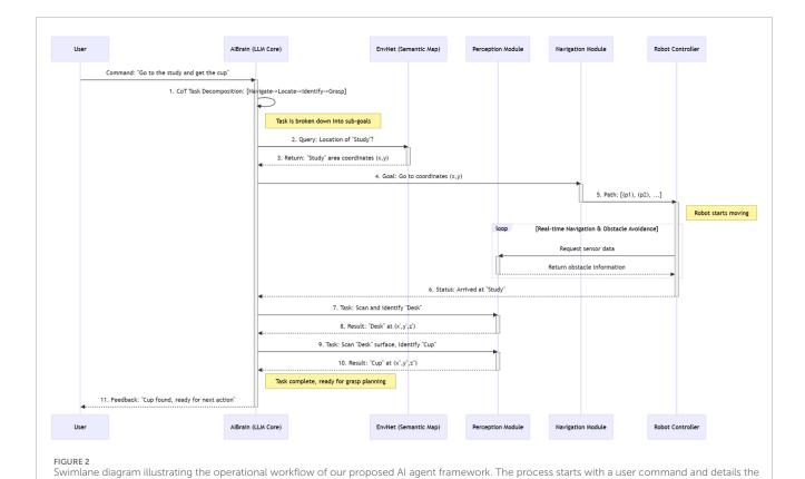
sequential interaction between the AlBrain, EnvNet, and RoutePlanner modules to achieve the final robot action. This visualization highlights the
