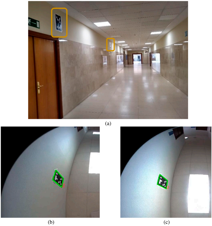
FIGURE 14 (a) Illumination challenges in a corridor scenario. (b) Correct detection of marker number 2. (c) Incorrect recognition of marker number 4.
