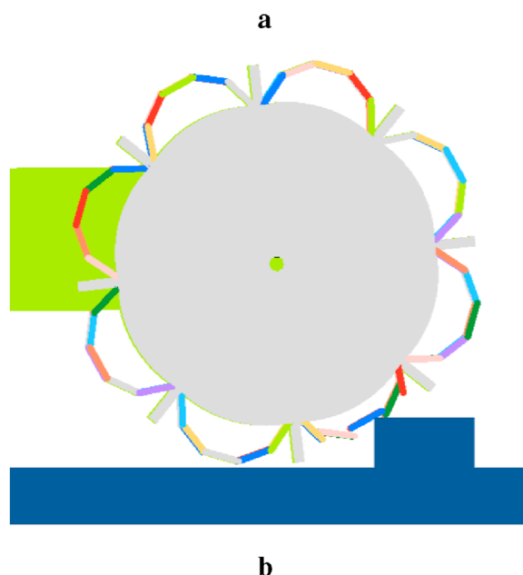
FIGURE 5 Comparison of the prototype and simulation at a key moment during traversal of a 15 mm high, 30 mm wide obstacle. (a) physical prototype (b) simulated prototype.
