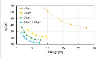
FIGURE 1 Timing resolution as a function of the collected charge from EXFLU1 LGAD sensors with different thicknesses: 45  $\mu m$  (orange circles), 30  $\mu m$  (yellow squares), 20  $\mu m$  (green triangles), and two 20  $\mu m$  sensors (blue diamonds). The error bars are not displayed.
