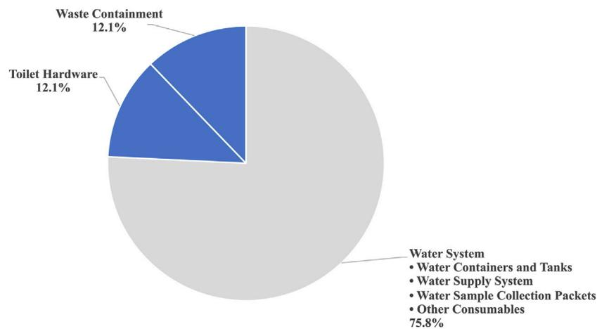
FIGURE 2 Mass breakdown of supplied items with regard to water recovery systems.
