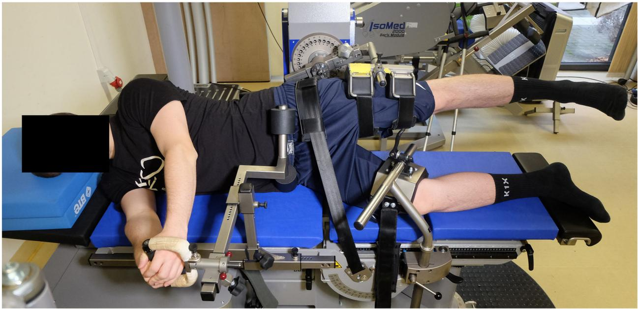
**FIGURE 3** | Set-up of the IsoMed 2000 dynamometer and participant positioning for the hip strength testing.
