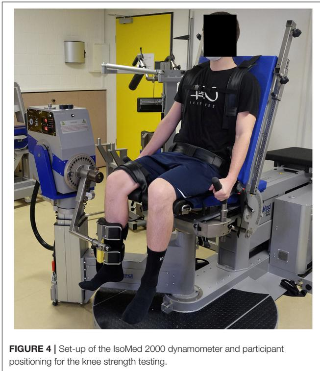
**FIGURE 4** | Set-up of the IsoMed 2000 dynamometer and participant positioning for the knee strength testing.
