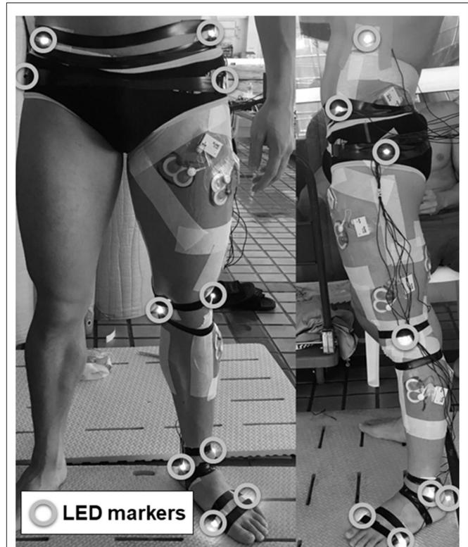
**FIGURE 1** | Images of a swimmer's left lower limb with active LED markers attached to 13 anatomical landmarks and surface EMG devices attached to eight muscles. Left: front view; right: lateral view.
