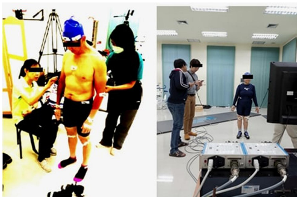
FIGURE 2 Marker placements on anatomical reference points used for motion capture.
