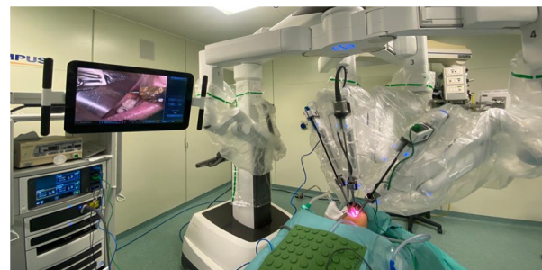
FIGURE 1 The Da Vinci Xi robotic system docking phase—the camera is inserted into the middle arm, then the two instruments (spatula and Maryland forceps) in the side arms.
