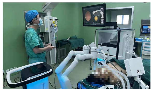
FIGURE 1 Thoracic surgeon operates bronchoscope robot for lesion localization.
