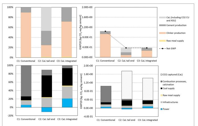
FIGURE 6 | GWP20 contribution analysis and relative emissions of the systems analyzed per kg of cement produced by the different phases (upper panels) and type of processes (lower panels) of the entire cement production cycle.
