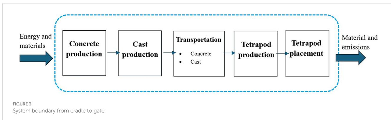
FIGURE 3 System boundary from cradle to gate.
