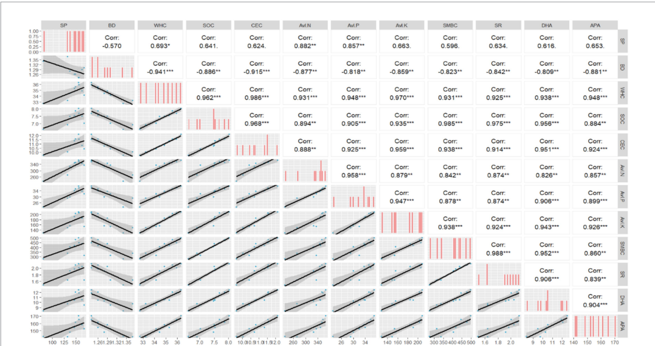
FIGURE 4 Correlation graph among soil physical, chemical and biological properties with system productivity (mean of 2 years). SP, system productivity; BD, bulk density; WHC, water holding capacity; SOC, soil organic carbon; CEC, cation exchange capacity; Avl-N, soil available N; Avl-P, soil available P; Avl-K, soil available K; SMBC, soil microbial biomass carbon; SR, soil respiration; DHA, dehydrogenase activity; APA, alkaline phosphatase activity. *Significant at the 0.05 level; **Significant at the 0.01 level; ***Significant at the 0.001 level.
