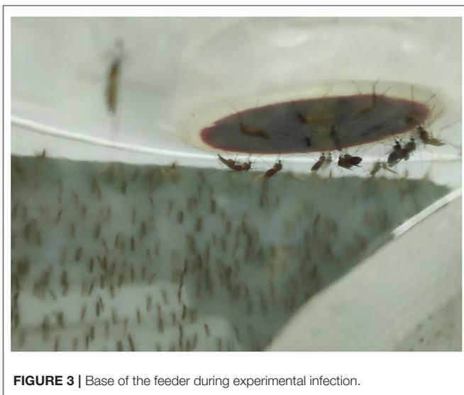
farmed quails) obtained from a local abattoir (**Figure 3**). The blood was pre-warmed to 41°C in a water bath (model SW22, Julabo, Germany), which was also employed as a hot water source to keep the blood warm inside the device. The circulation of water between water bath and device and vice versa was achieved with a small water pump (CompactON 300, Ehein, Germany) connected to the feeding device by rubber hoses.
