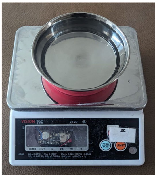
FIGURE 3 Displaying a custom-built scale that had an accuracy of 1 g and recorded weights every 5 s in Experiment 1 and every 30 s in Experiment 2. Scales were calibrated using a 2,000 g calibration weight and regression coefficients were applied to each scale to ensure precision in measurements.
