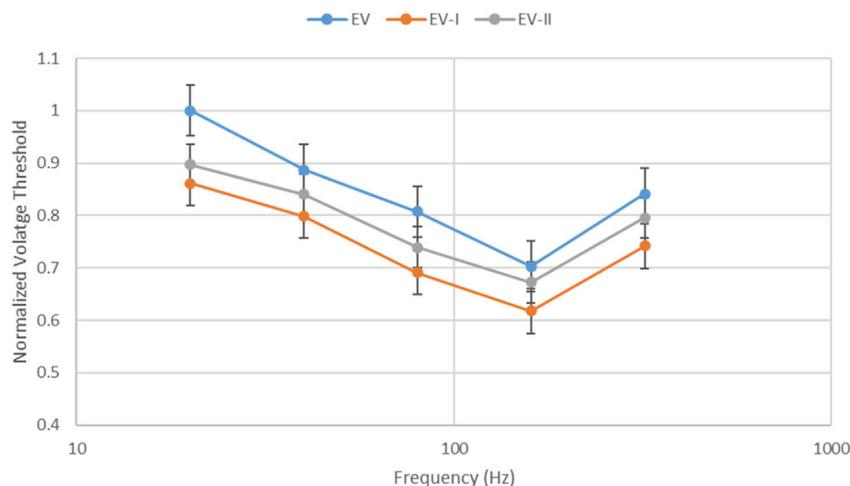
FIGURE 7 Average threshold curve (normalized) for electrovibration and the reduced threshold when background electro tactile stimulus is presented together on subthreshold.
