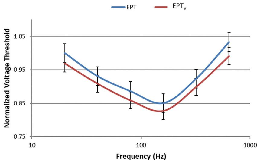
FIGURE 6 Average threshold curve (normalized) for electro tactile stimulus and the reduced threshold when skin temperature is raised by seven.
