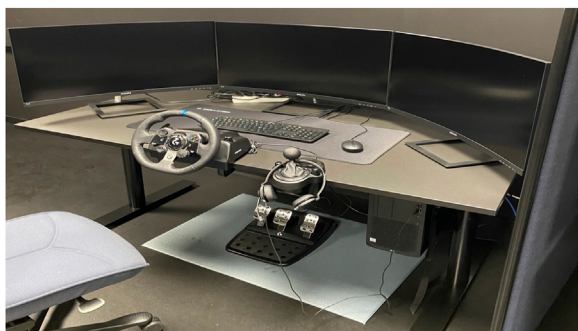
FIGURE 1 Three-monitor simulator configuration with steering wheel and pedals.
