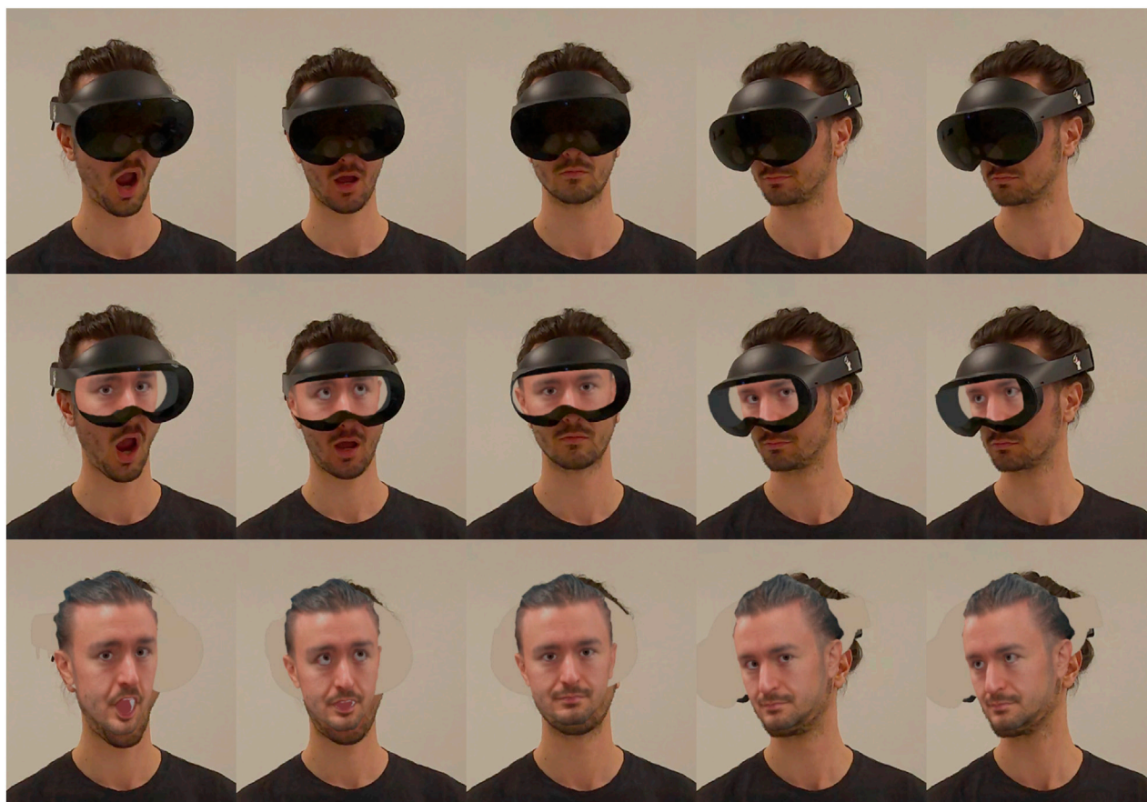
FIGURE 1 Co-located headset wearer viewed by another headset wearer ( top row ) is blended with their aligned avatar, either via our “see-through visor” ( center row ) or as “head substitution” ( bottom row ). See Supplementary Video for demonstrations of all conditions in varied poses.
