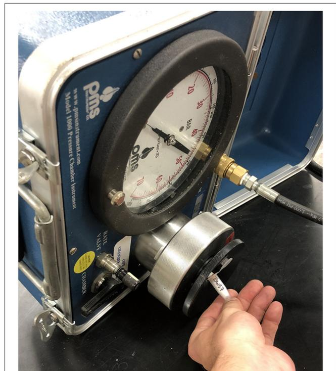
**FIGURE 2** | Example of collecting Stem-PC sample into Eppendorf tube filled with glass wool and the PMS instruments Model 1000 pressure chamber instrument on its side so that gravity helps facilitate the collection of sap.
