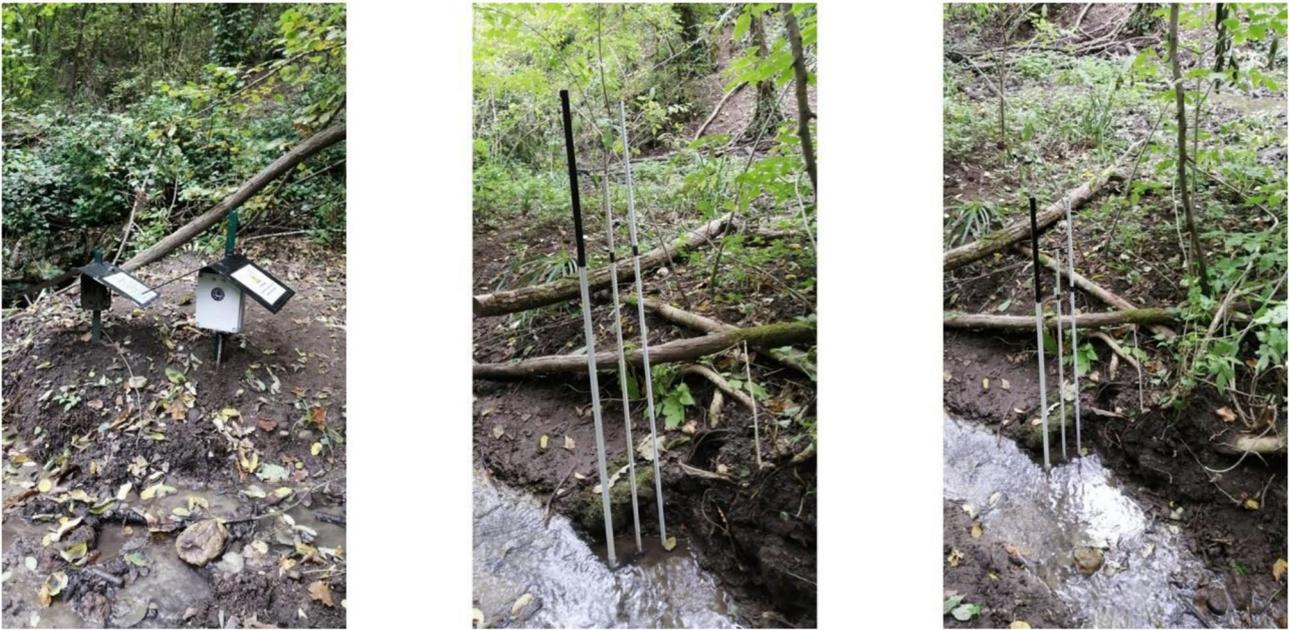
FIGURE 1 An example of stage-cam system installed at the Montecalvello basin.
