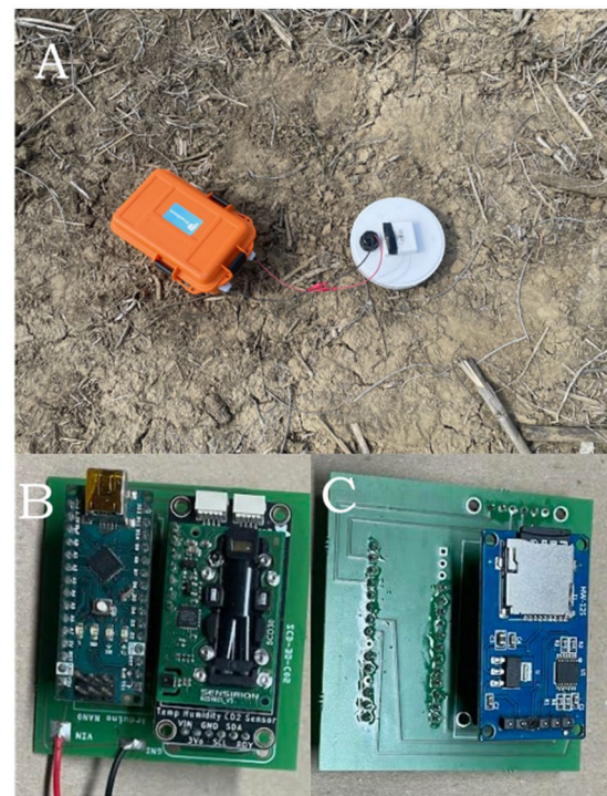
FIGURE 1 V1 sensor deployed in the field. The orange box is the battery box and the white PVC is the chamber (A). V3 sensor top (B) and bottom (C) including, from left to right, the Arduino Nano, Adafruit SCD-30, and SD card reader.
